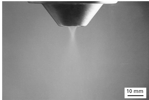
Figure 4 A view of cone-shaped powder stream.
