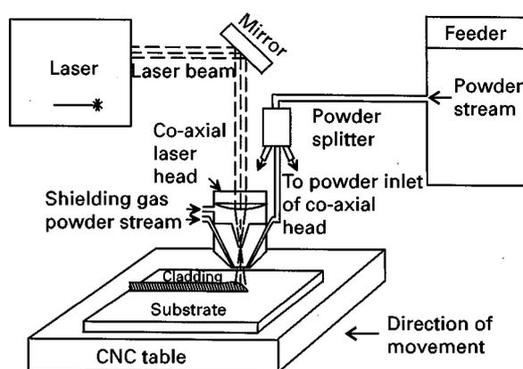
Figure 1 A schematic drawing of the laser cladding system.
