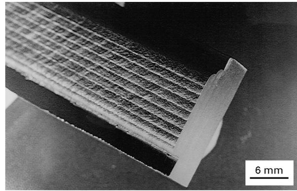
Figure 7 A top view of LMMC sample with smooth surface, no macroscopic cladding defects, and sharply discrete interface via laser cladding (Sample C).
