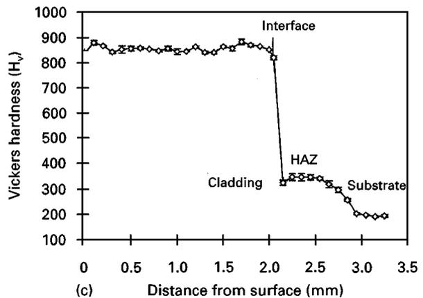
Figure 10 Microhardness profiles of sample E: (a) as-clad, (b) as-clad + tempering, (c) as-clad + tempering + liquid nitrogen treatment.
