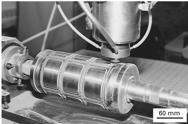
Figure 6 Hard-facing tracks, with complex geometric patterns, deposited on a steel roller for fabricating a rotary cutting die by the laser cladding process (Sample B).
