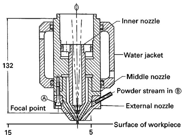
Figure 3 A schematic drawing of the transverse section of a coaxial nozzle. (A) 3 screw bolts, (B) 4 inlets. All dimensions in mm.
