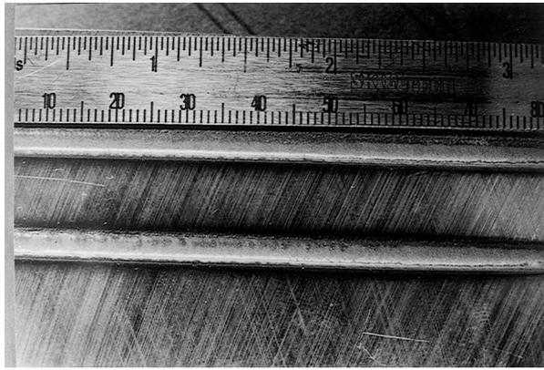
Figure 5 A view of single hard-facing cladding tracks with a smooth surface, uniform cladding thickness, and width (Sample A).
