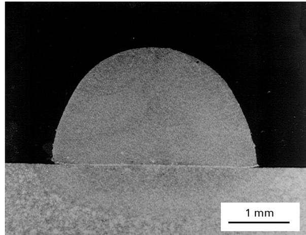
Figure 8 An optical micrograph of the cross-section of hard-facing tracks with no cladding defects (Sample D).
