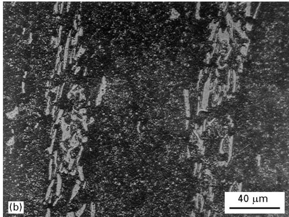
Figure 9 Overview of carbides in CPM 10V and D2 alloys. (a) Fine vanadium carbides uniformly dispersed in the matrix in CPM 10V tool steel (Sample E). (b) Segregation and blocky carbide morphology in D2 alloy.
